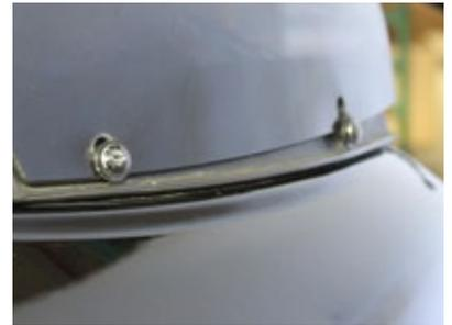
3. Install your new Flare™ Windshield onto the mounting screws. Torque the two center screws first, then the two outer screws.
