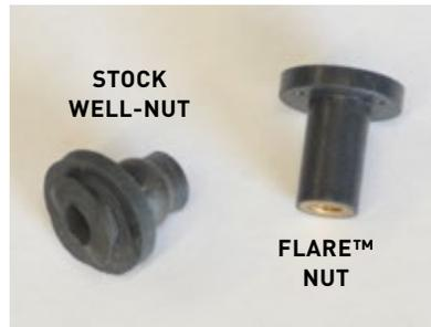
2. Check the well-nuts in the fairing, if they are damaged or broken, Klock Werks offers a replacement kit (part number 2404-0548) for \$29.95
